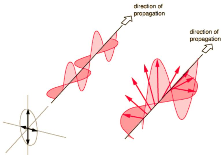
Figure 2.1.2: Elliptical Polarization
