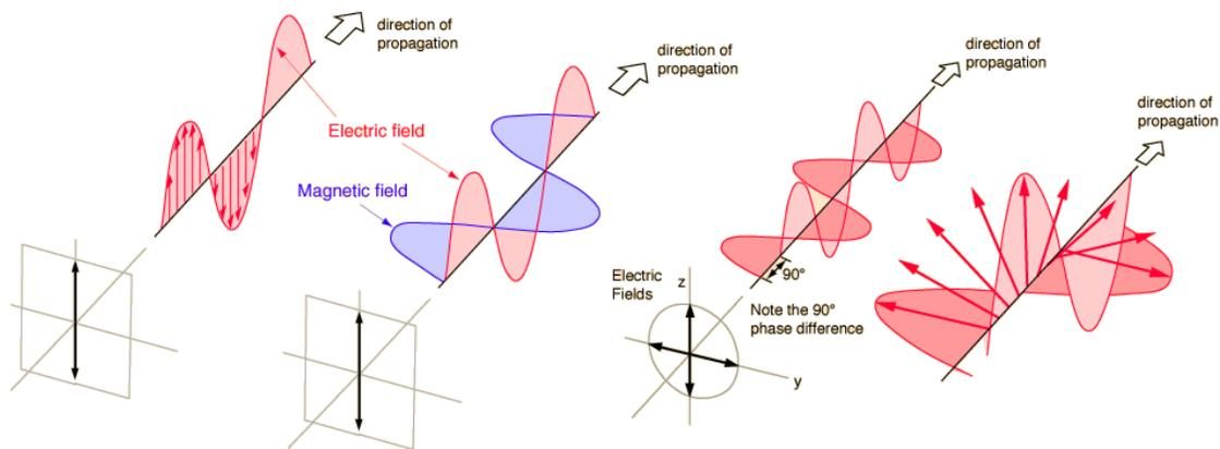
Figure 2.1.1: Linear and Circular Polarization
