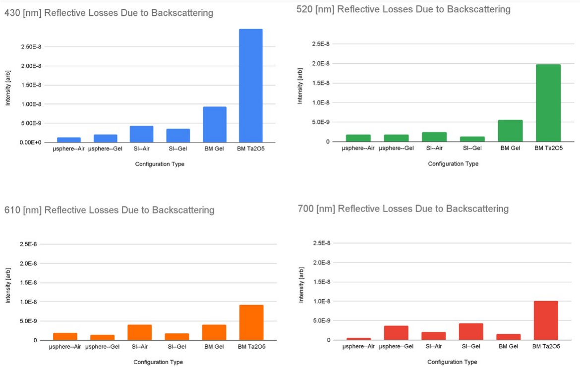
Figure 6.3.14: Reflective losses due to backscattering. Backscattering is considered within the 344\text{--}16^\circ range. Plot colors organized by corresponding visible wavelength. Each configuration had an overall radius of 5 microns. Synthetic iridocytes both had constituent nanoparticles of diameter 250 [nm]. Both Bragg mirrors had quarter wavelength thickness corresponding to 520 [nm].
