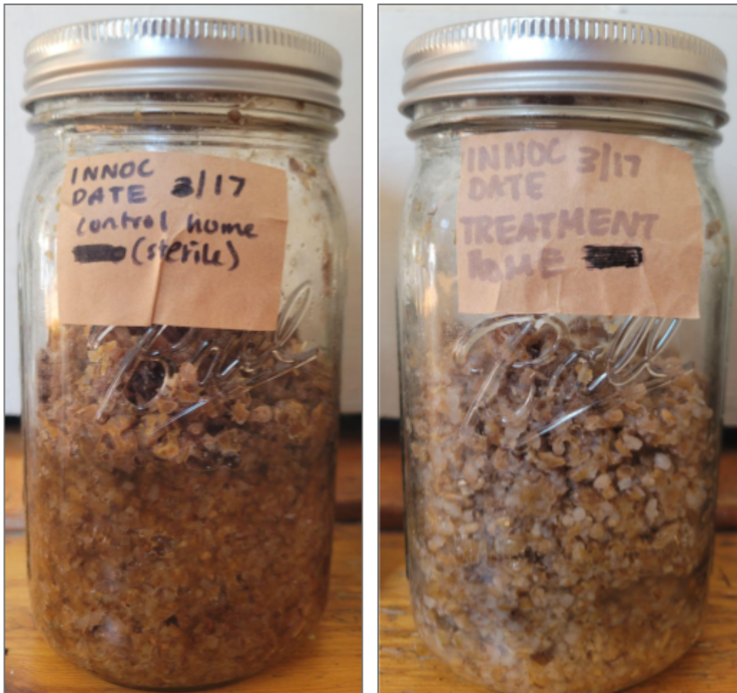
Fig. 3. Spent grains from the homebrewing process 35 days after inoculation with fungal liquid culture. From left to right: sterilized homebrewing sample, unsterilized homebrewing sample.
