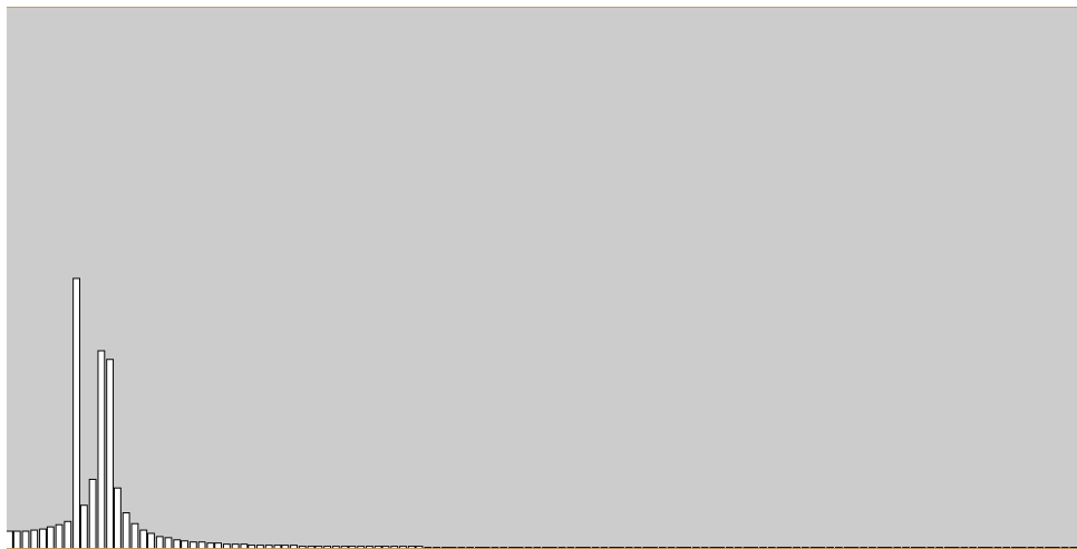
Figure 2.5.3. Amplitude spectrum for x[t] = -\cos(\frac{16\pi t}{256}) + \sin(\frac{23\pi t}{256}) . Clearly we see a peak at 8Hz, 11Hz and 12Hz.
