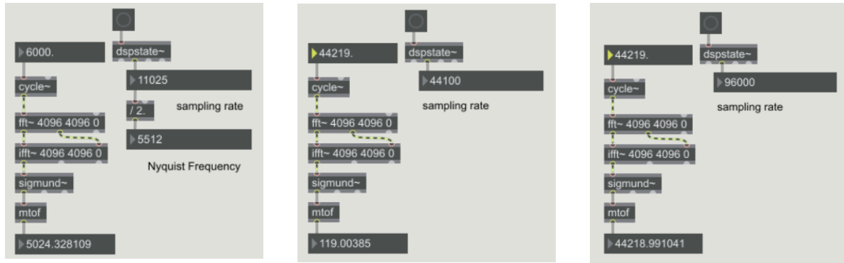
Figure 2.0.4. Frequency aliasing based on sampling rate
