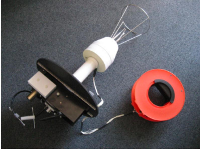
Figure 2.3.1: SCAMP pictured. The scanners are the three prongs guarded by the cone-shaped cage. Below are the wooden floats used to regulate the instrument's buoyancy. The circular bottom section allows SCAMP to glide downwards at an angle to avoid measuring its own wake as it rises to the top. Lastly the string attached to the orange wheel serves to reel SCAMP back in after it has surfaced.
