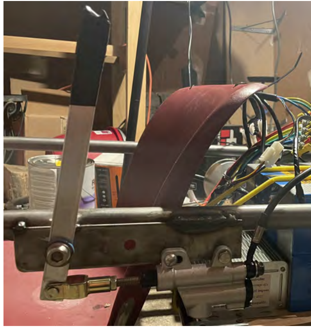
Figure 3.2.9: Hand brake, displaying master cylinder
