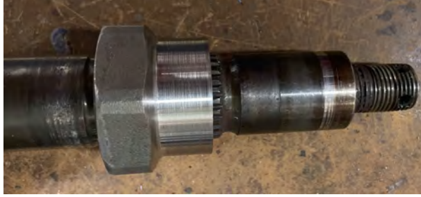
Figure 3.2.7: Hub splines after reducing diameter; fitment to axle end
