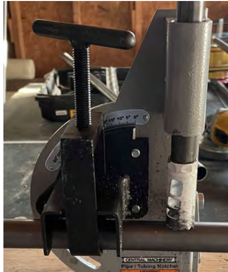
Figure 3.1.3: Tube piece set into notcher, display shows the ability to change the cut angle.
