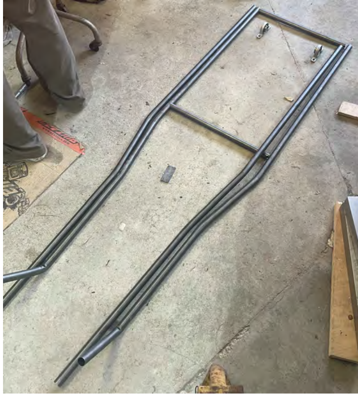
Figure 3.2.1: Lower and upper frame tubes after bending, laid out to match up bends
