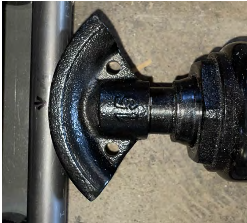
Figure 3.1.1: Tube section mounted in Hydraulic press, marking indicates the bend point.
