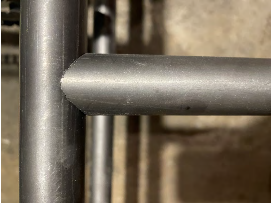
Figure 3.1.2: Fit of a notched tube to adjoining section
