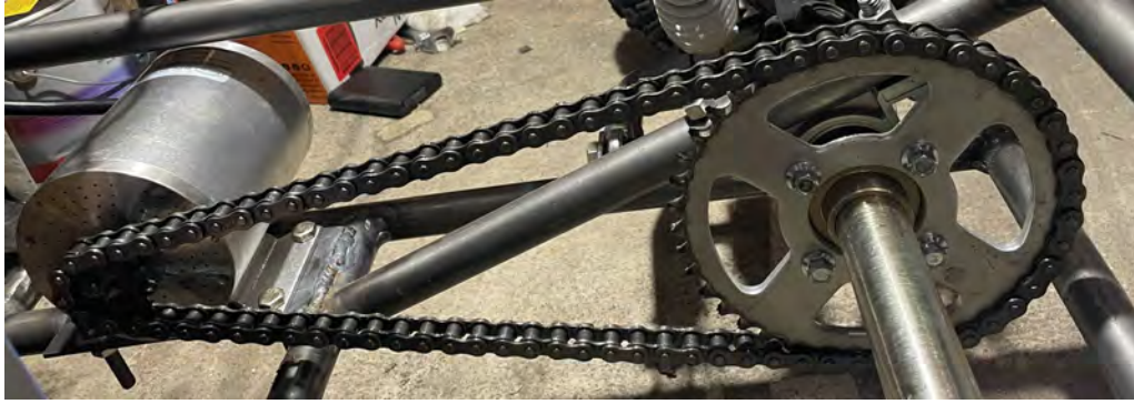
Figure 2.2.3: The chain drive setup of the vehicle, displaying the sprocket size between driver and driven
