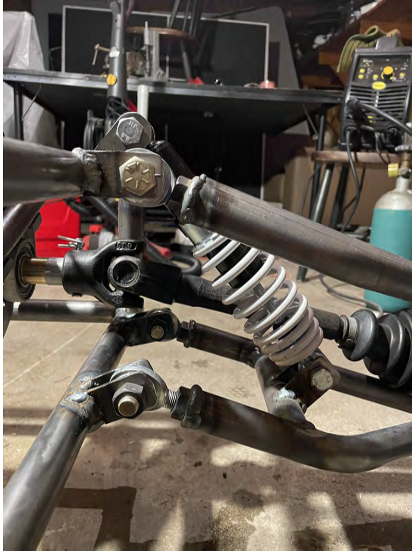
Figure 3.2.4: Swing arms connection to frame; bolted to suspension brackets using rod end to allow arms to rotate about fixed point.
