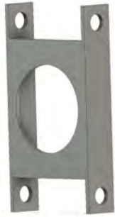
Figure 1: The rear wheel hub holds a bearing for the axle shaft to be connected to wheel. Two bolts are used to fix the top and bottom to the ends of the rear swing arms
