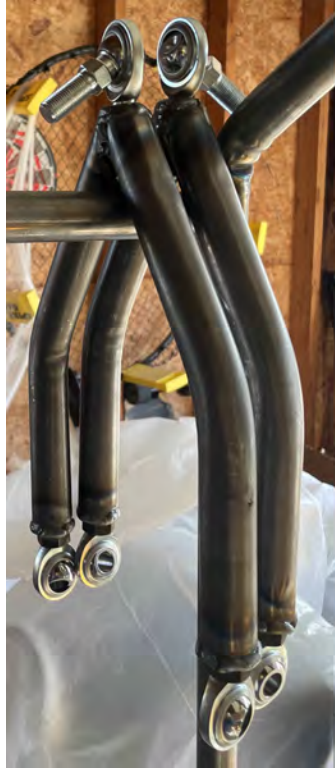
Figure 3.2.3: A completed front swing arm; the rod ends at the bottom are those previously described, at the other end a tie rod end is welded. Tie rod ends allow for rotation and sweep an angle that will allow the swing arms to move vertically while keeping the wheel parallel to the surface of travel.
