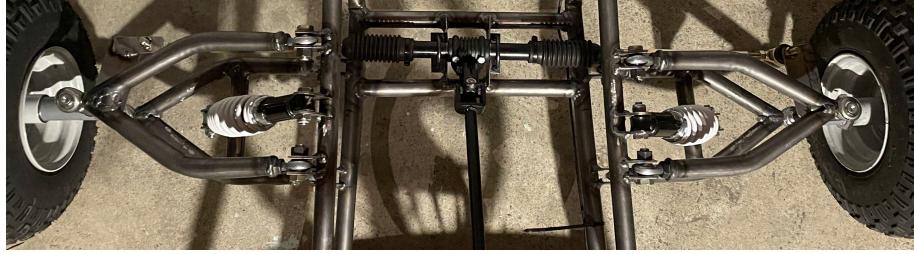
Figure 3.2.5: Steering system mounted on vehicle, showing connecting brackets for wheel hubs and rod ties.
