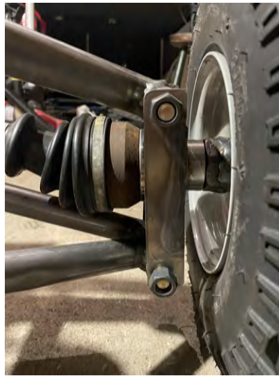
Figure 3.2.8: Final assembly of axle shaft held by wheel hub and bearing. The connection to wheel using splines from original vehicle
