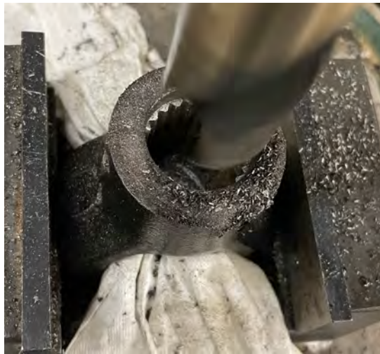
Figure 3.2.6: Removing splines for connection to Drive Shaft
