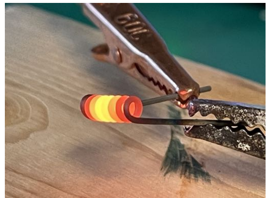
Figure 2.49: The glow of the filament at 24A
