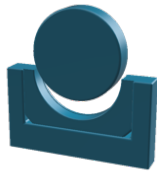
Figure 2.18: The jig used to curve the back face for the half-moon plate
