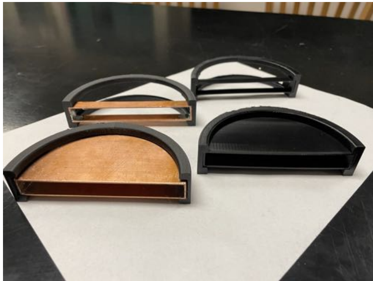
Figure 2.23: The electric plate in the mounting system
