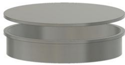
Figure 2.27: Concept design of aluminum vacuum chamber
