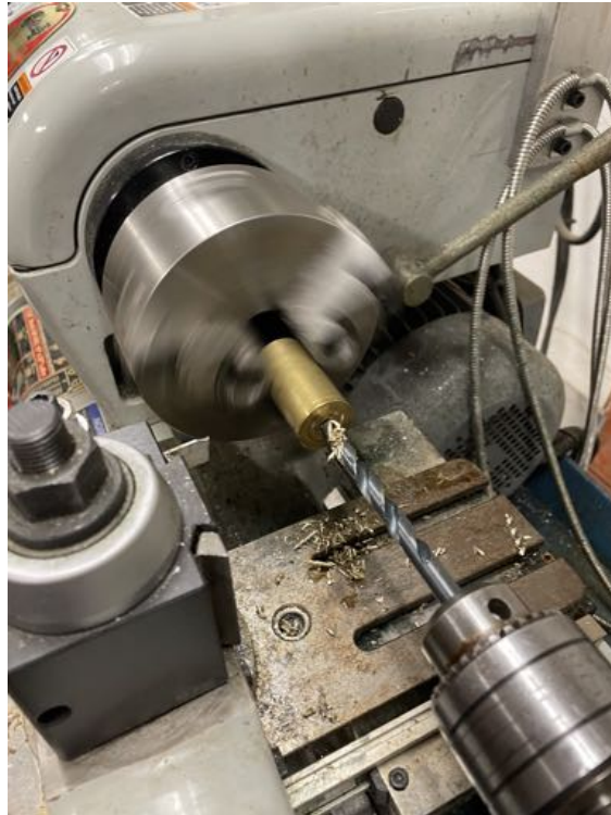
Figure 2.57: The Process of Hollowing Out the Center of the FC
