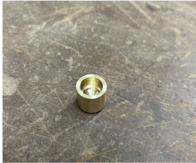
Figure 2.58: A Finished Version of the Faraday Cup
