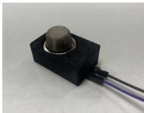
Figure 2.45: The sensor in the protective box
