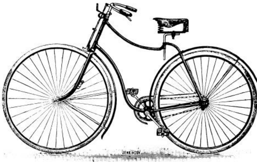
Figure 5. “Starley” brand safety bicycle. This style of bicycle, the progenitor to modern bicycle designs, was the first of its kind. Ushering a new era in bicycle use throughout the world, its design was safer and easier to use than previous iterations.
