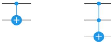
Figure 3.1.5: Circuit diagram representation of the controlled-NOT and Toffoli gate respectively [9].
