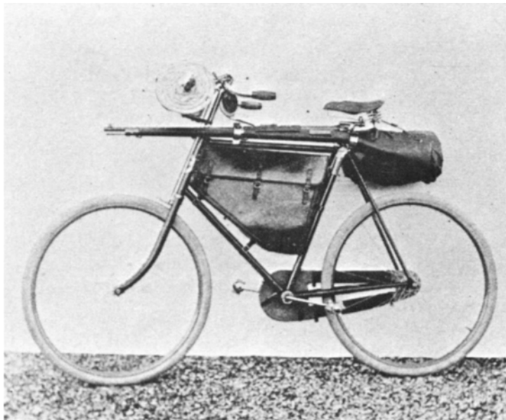
Fig. 17 A fully loaded military bicycle, including a bed roll, provisions, a custom frame bag, and a mount for a rifle 58
