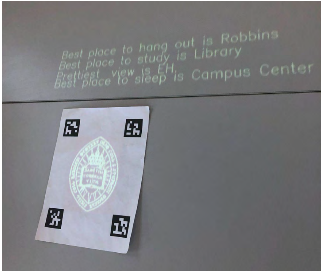
Figure 23. After traceMode.py is executed, the results of the detected colors are projected when the second ArUco screen is placed in the frame. (Author's Photo, 2022)
