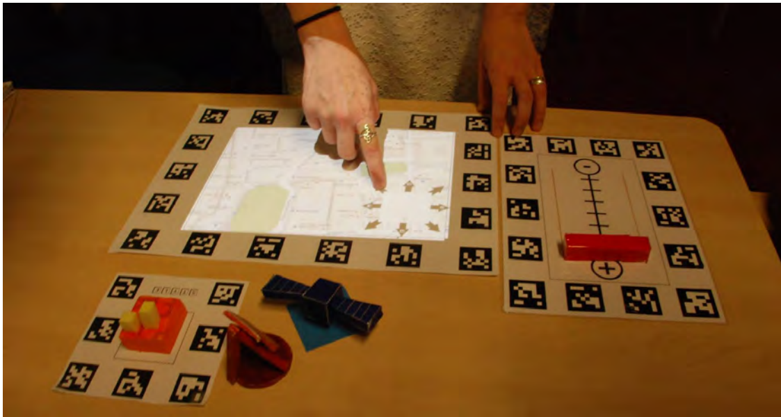
Figure 3. Hand gestures and objects are used to interact with SyMAPse, and multiple sheets of paper can be used in these interactions [12]
