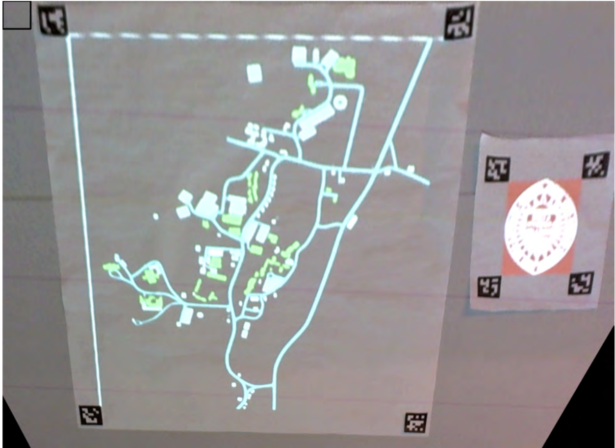
Figure 13. Warped perspective on the homogCamToComp homography matrix (Author's Photo, 2022)
