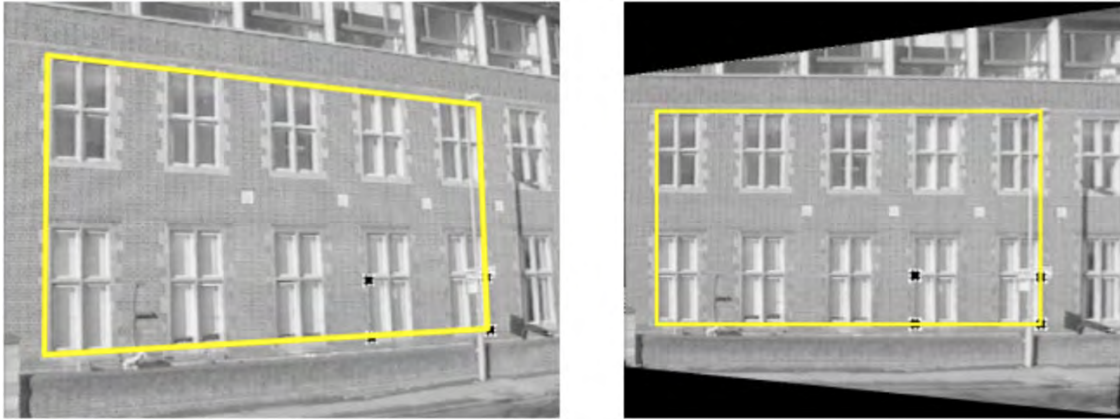
Figure 9. Two images taken from different angles where a homography matrix is determined [14]
