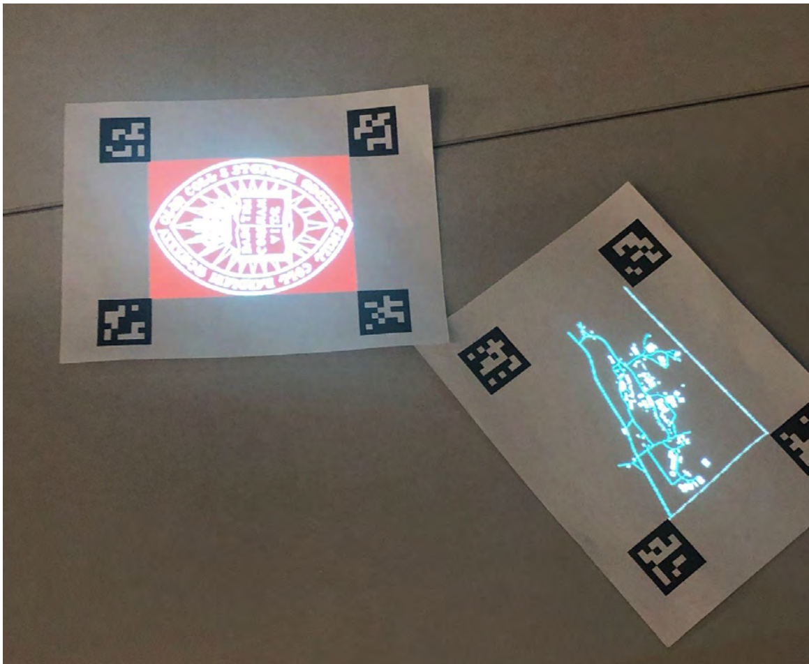
Figure 15. ArUco B projecting the Bard logo (left) and ArUco A projecting the campus map (right) (Author's Photo, 2022)
