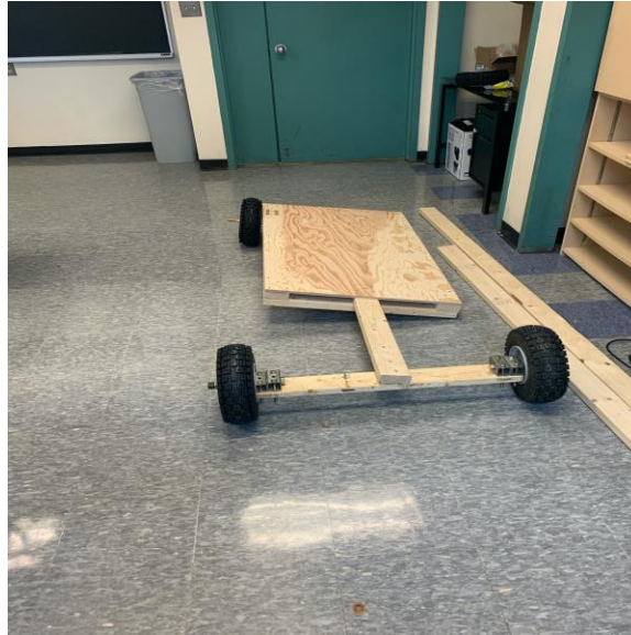
Figure 3.1.1 Depiction of how steering plank connects the kart 1
