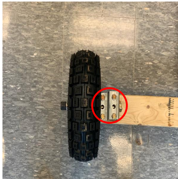
Figure 3.2.1 Wheel mounted onto the steering plank using galvanized steel rail.
