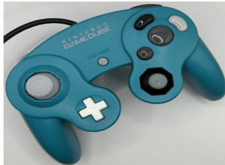
Figure 3: A customized controller with a notched left stick, and unnotched right stick. 70
