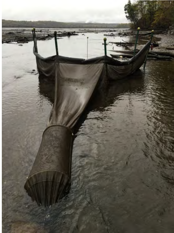
Fig. 4. The fyke net installed at the mouth of the Saw Kill as it enters Tivoli Bays at low tide
