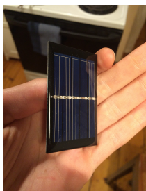
Figure 3.2.1. A front view of one of the miniature solar cells I first purchased from P&T Surplus. The dark blue strips are the photovoltaic material, and are shielded by resin.
