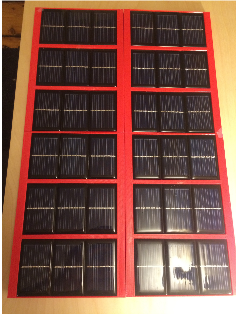
Figure 3.4.1. The 6x6 solar array that I created for the purpose of charging an iPhone. Each set of three cells is connected in series, and all twelve sets of three are connected in parallel. A complicated design for the tunnels which run throughout the board was required to allow for this wiring to be done correctly. The array comes in four separate pieces, because the whole thing was far too large to be 3D printed all at once.
