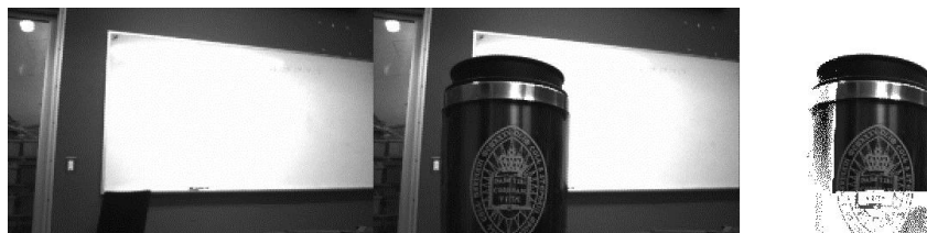
Figure 4.3.4: Images Taken using the Background Subtraction Program. In order from left to right; old, new, result
