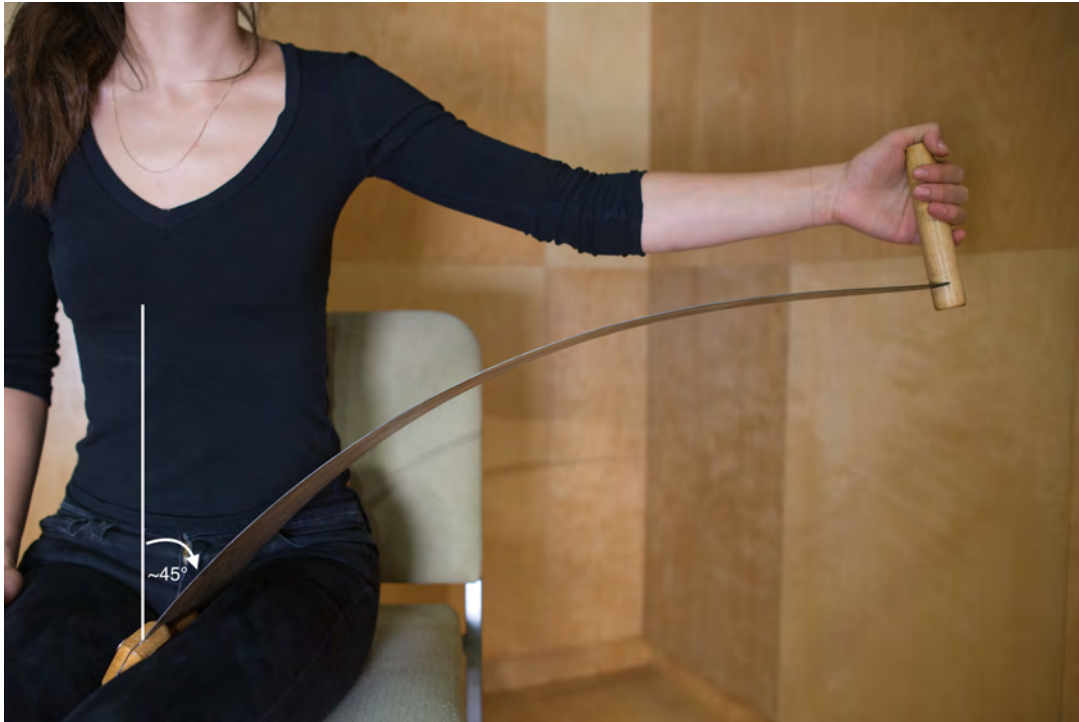
Figure 8: Forming the first arch.
